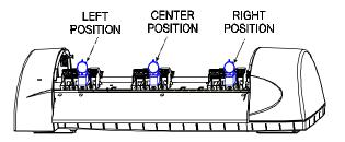
Figure 3-20. Carrier Positions for Head Height Adjustment.
